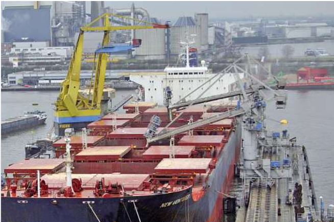
Fig. 1: Bulk handling by the means of screw conveyors.
