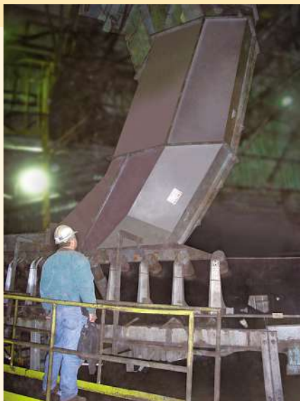
The flow-engineered chute technology reduces spillage and extends conveyor belt life.
