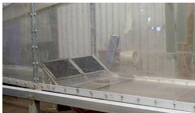
Fig. 3: The wind tunnel test tray holder and trays at 37°.
