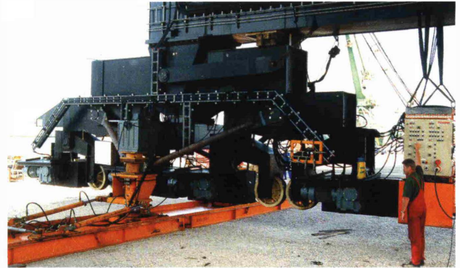
Fig. 3: Skidding in operation with the 'Air Cushion' system
