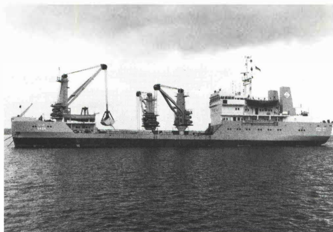
Fig. 1: Multi grab dredger "GAZA"
