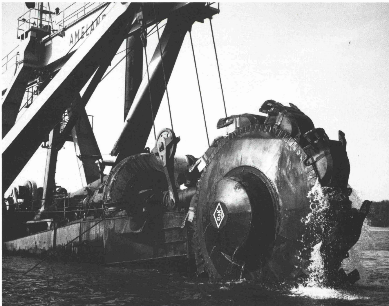
Fig. 6: Underwater bucket wheel — prototype
