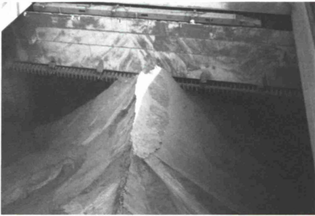
Fig. 3: First run of fixed screw, taking off tops.
