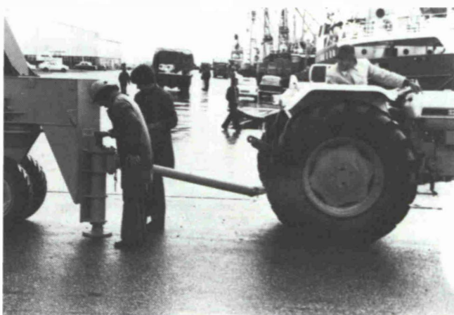
Fig. 3: The multi-port system can be operated by a towing vehicle. It can also be supplied with its own drive
