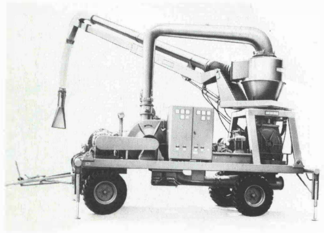
Fig. 6: Mobile conveyor with hydraulic telescopic boom
