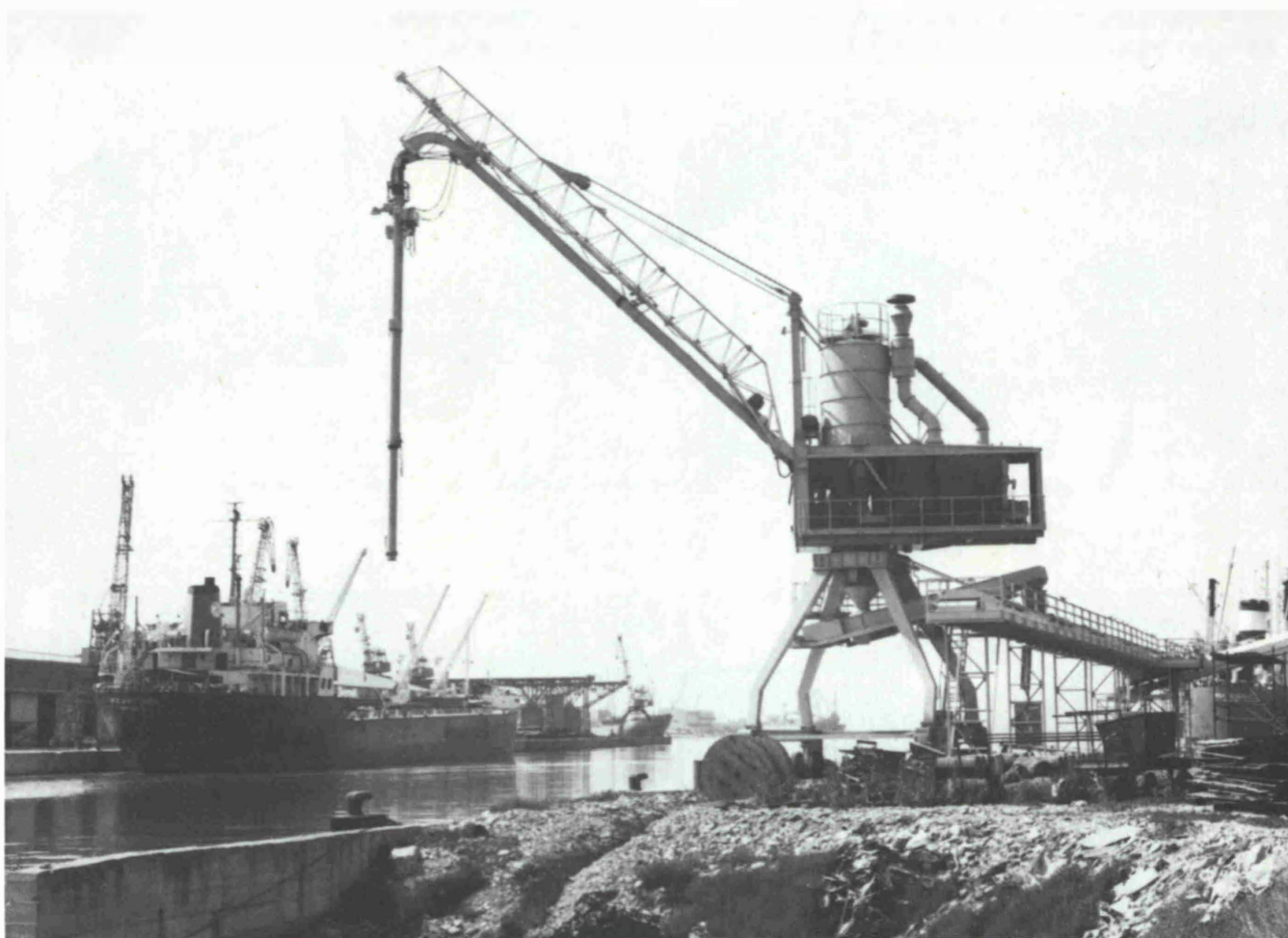
Fig. 2: Multi-port system for unloading sea-going ships (maximum conveying capacity about 280 t/h for grain)
