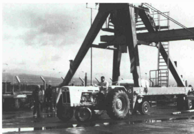
Fig. 3: The multi-port system can be operated by a towing vehicle. It can also be supplied with its own drive
