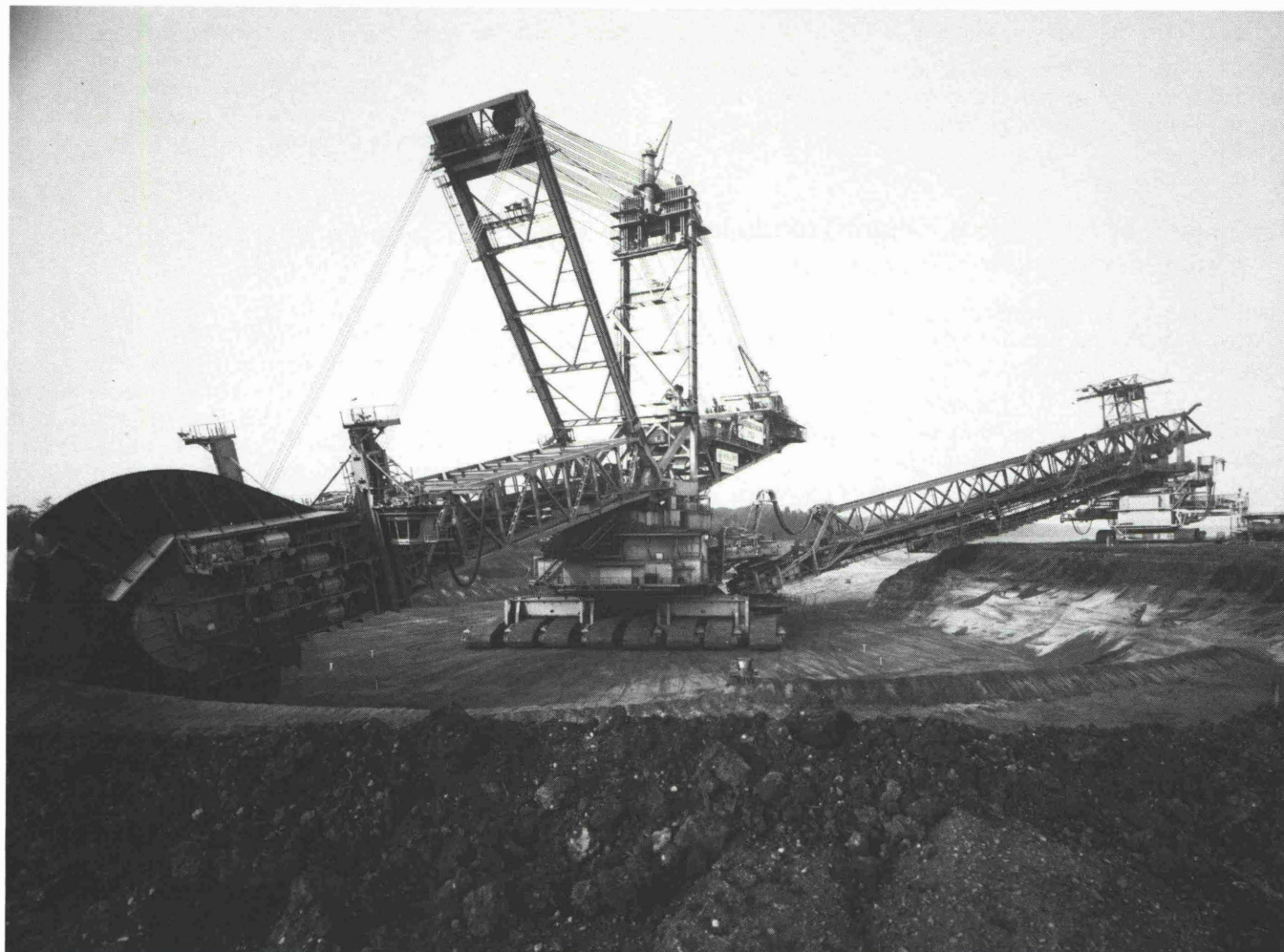
Fig. 1: Bucket-wheel excavator with a capacity of 240,000 \text{ bank m}^3/\text{day}
