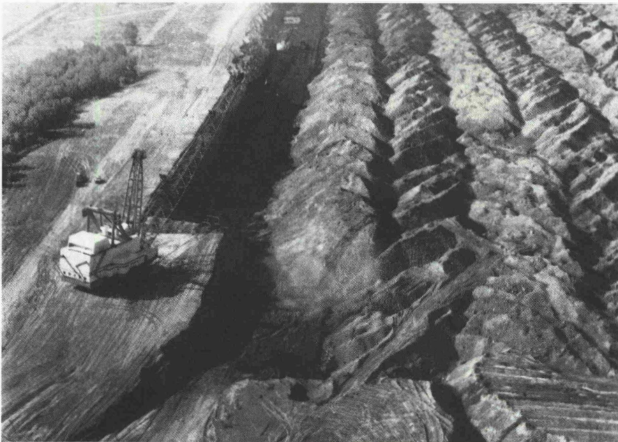
Fig. 1: Typical strip mining operation with dragline
