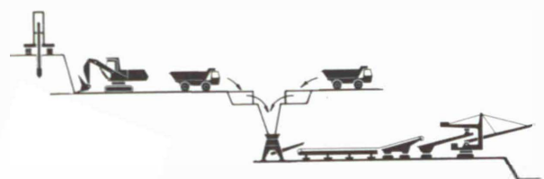
Fig. 5: Combined mining system with intermediate truck haulage and mobile crusher
