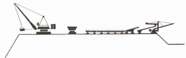
Fig. 6: Discontinuously working dragline feeding material via hopper car onto belt conveyor
