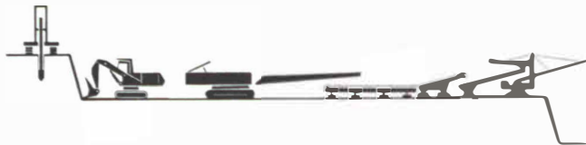
Fig. 8: Grading by hopper belt wagon prior to feeding onto conveyor
