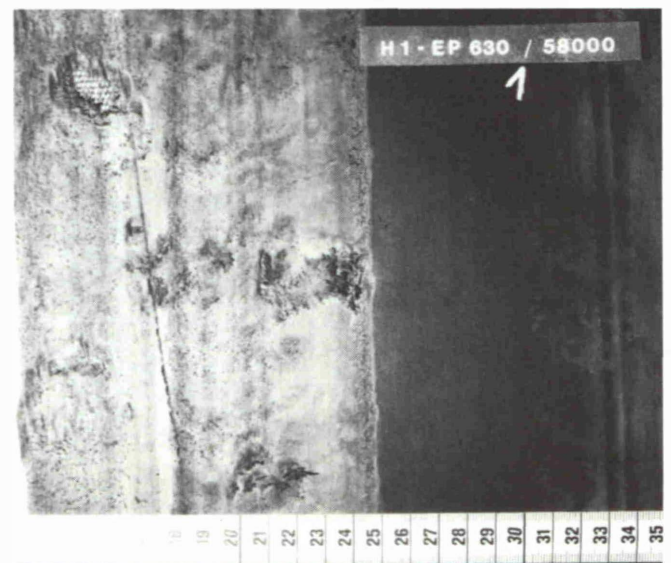
Fig. 3: Wear occurring in a steelcord belt ST630 after 31,225 rotations on the test stand
