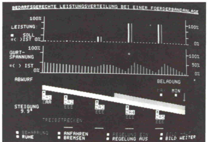
Fig. 6: Belt tension plotting and load-dependent power distribution of a belt conveyor with controlled drives (compare Fig. 2).
