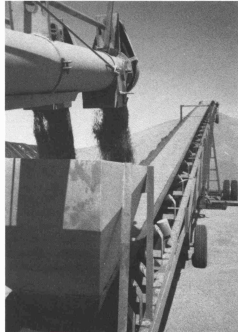
Fig. 2: Portable unloading equipment showing the 100 ft, 200 t/h conveyor belt
