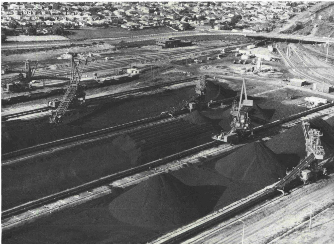
Fig. 1: Stockpile arrangement of Port Waratah Coal Export Facility, showing PWH bucket wheel reclaimers and stackers
