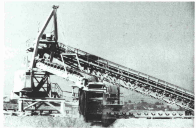
Fig. 5: Height of free-fall minimised to prevent undue dust loss
