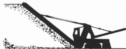
Crawler-mounted scraper for reclaiming material from small stockpiles
