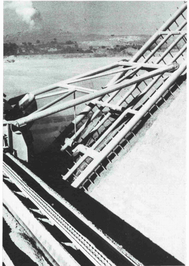
Fig. 11: Harrow arrangement on the bridge-mounted bucket wheel reclaimer
