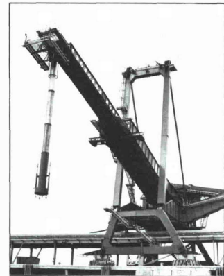
Fig. 5: Travelling shiploader with telescopic chute in extended position
