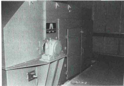
Fig. 5: Measuring room with elevator head and large observation opening
