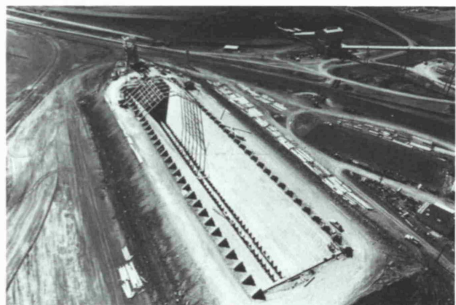
Fig. 9: Aerial view of 100,000 t storage slot at Cordero Mine
