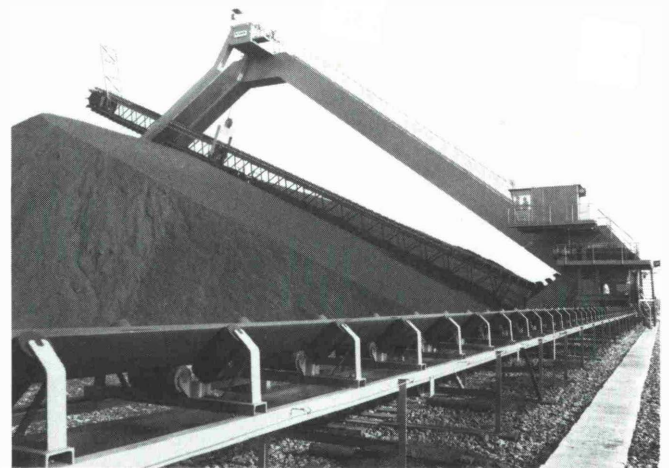
Fig. 3: Portal scraper reclaimer for coal blending — 50m span (Courtesy of Klöckner power station, Rauxel)
