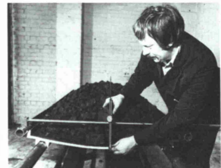
Fig. 2: Cross-section showing the belts parabola shape
