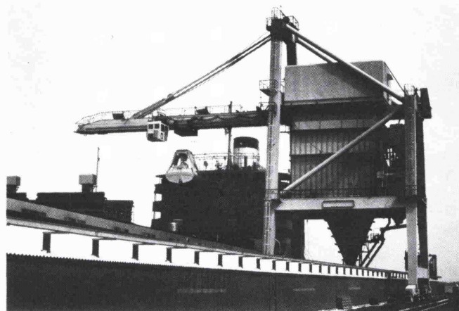
Fig. 1: A 1000 t/h grab bucket unloader. The machine features a semi-automatic operation mode and an integrated dust collection system, and is used exclusively to unload alumina
