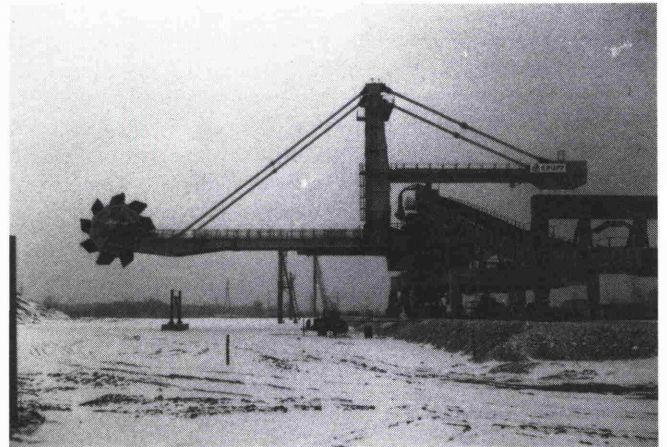
Fig. 13: Stacker/reclaimer for 4,000 ton/h stacking and 3,600 ton/h reclaiming of coal for Detroit Edison
