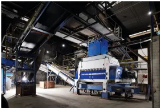
High-throughput secondary shredding: Lindner's Komet Series 3 (Pictures: © Lindner-Recyclingtec GmbH)
