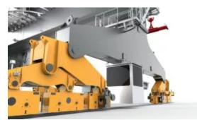
Among the crane's unique features is an observer cabin attached near the tracks at the bottom of the crane. This provides another layer of supervision for additional workers to keep an eye on the crane's operations.
