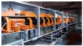
Martin Engineering transfer points are designed to create a safe and low maintenance sealed environment.
