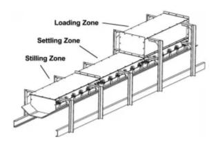
The Martin<sup>®</sup> Transfer Point Kit is a heavy-duty horizontal enclosure for the loading zone. Each kit is either ordered as a loading zone, settling zone, or stilling zone. The width and length of the kit are determined by the receiving belt's width and speed and the dust characteristics of the material being transferred. Dustier applications may require a longer settling zone.
