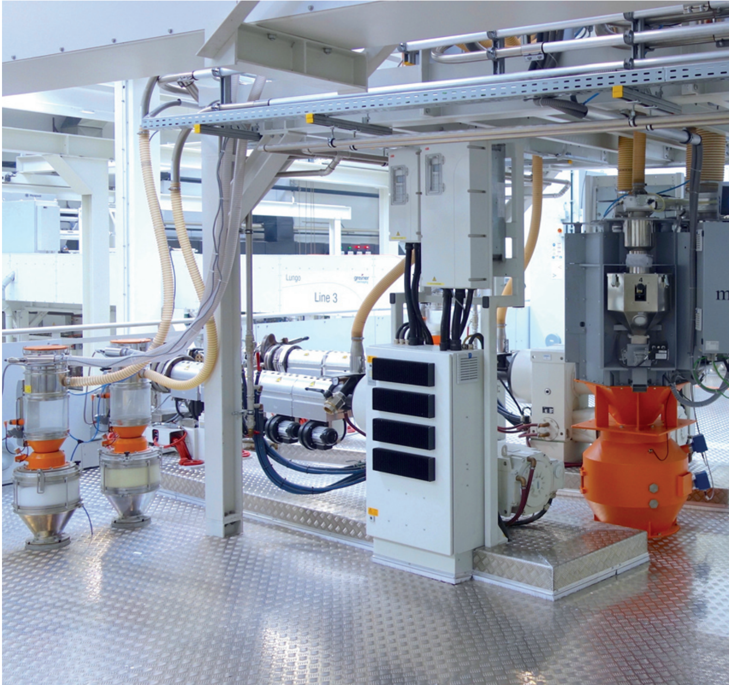
Fig. 5: Central mixing station to supply the “regrind extruder”. In this, four material components come together (regrind from the silo or from the BigBag, stabiliser for the adhesion promoter and new PP material) which are added from the gravimetric dosing
