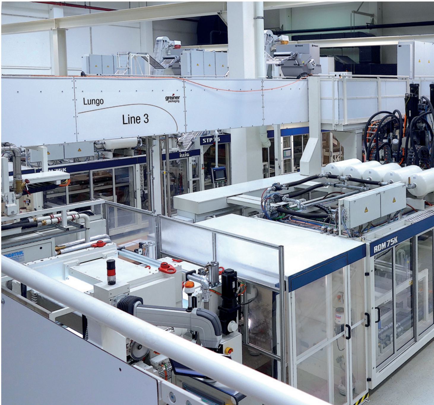
Fig. 2: The 7 layer barrier foil which comes out of the extrusion machine runs directly into a multi cavity deep drawing and punching machine. The remaining punched frame and any bad parts produced are then fed directly into a cutting mill (in the background at the end of the machine) and fed back into the production line from there.
