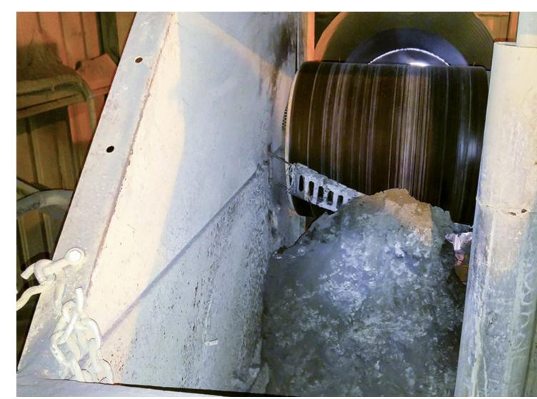
Mounted diagonally, commonly at a  $17^{\circ}$  angle, the CleanScrape spans the entire belt profile.
