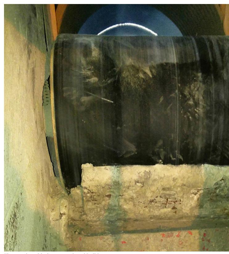
The previous blade accumulated buildup and encrusted material, degrading cleaning performance.
