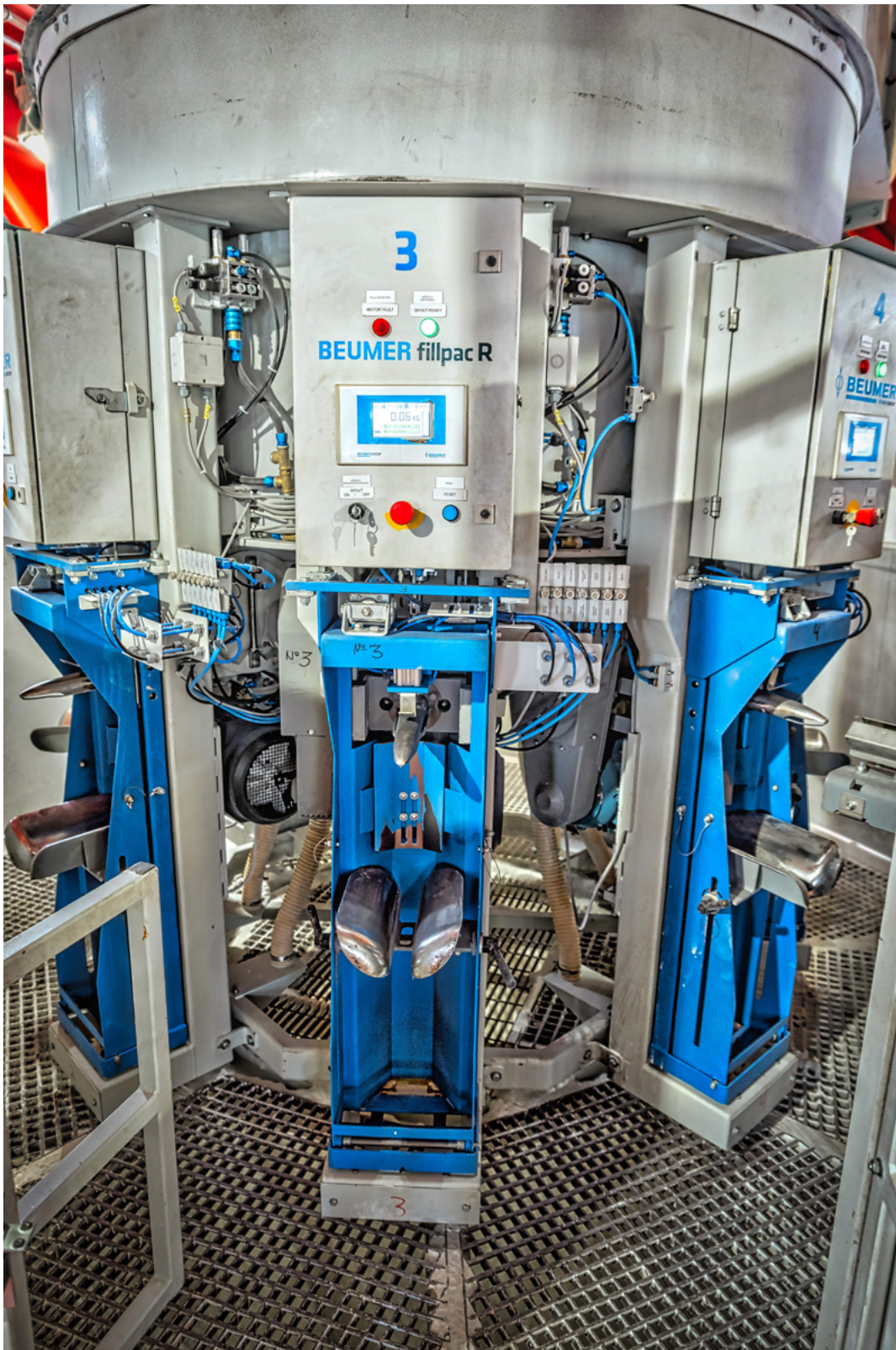
Picture 3: BEUMER Group supplies everything from one single source. This includes the BEUMER fillpac filling system. It can be adjusted to the changing parameters of the different materials.
