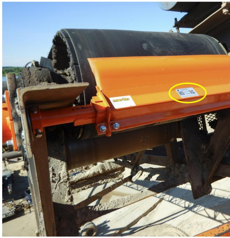
Martin Engineering has introduced data tracking and analysis codes on conveyor belt cleaners.
