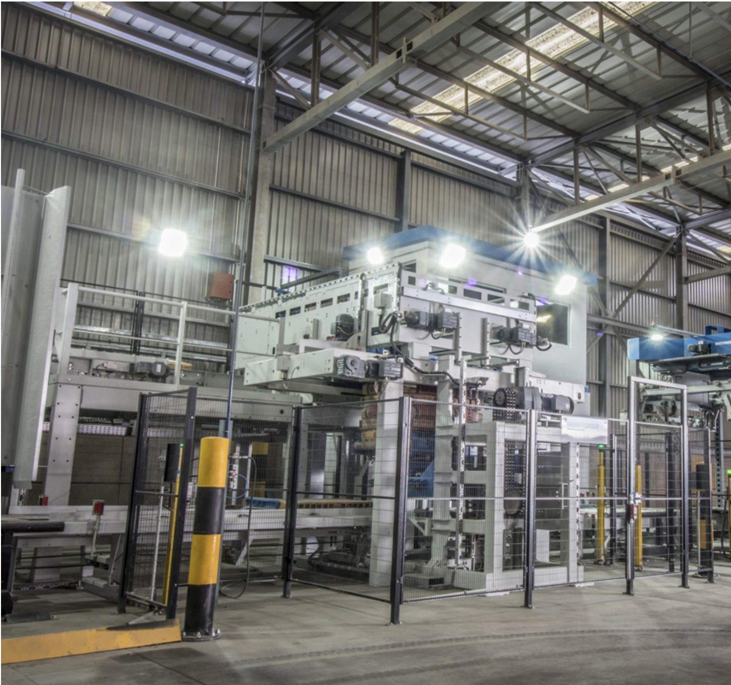
Picture 5: Palletising and packaging process: BEUMER Group supplied a BEUMER paletpac 3000 and a BEUMER stretch hood A.
