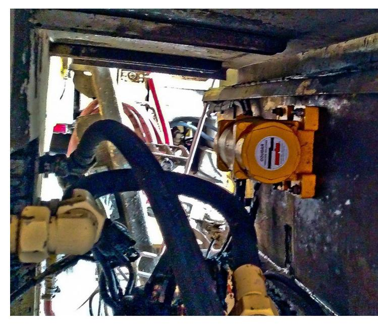
The MDC12 can be specified with a force output of 400 lbf (90 N) or 700 lbf (160 N) for larger applications.
