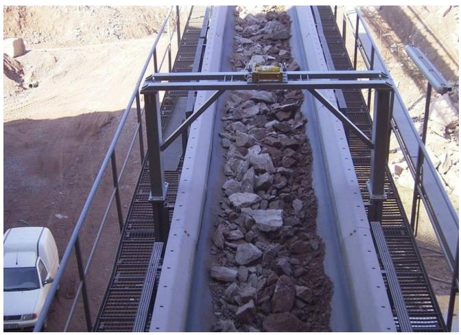
The non-contacting belt scale LB 472 can be installed directly after bunkers,
