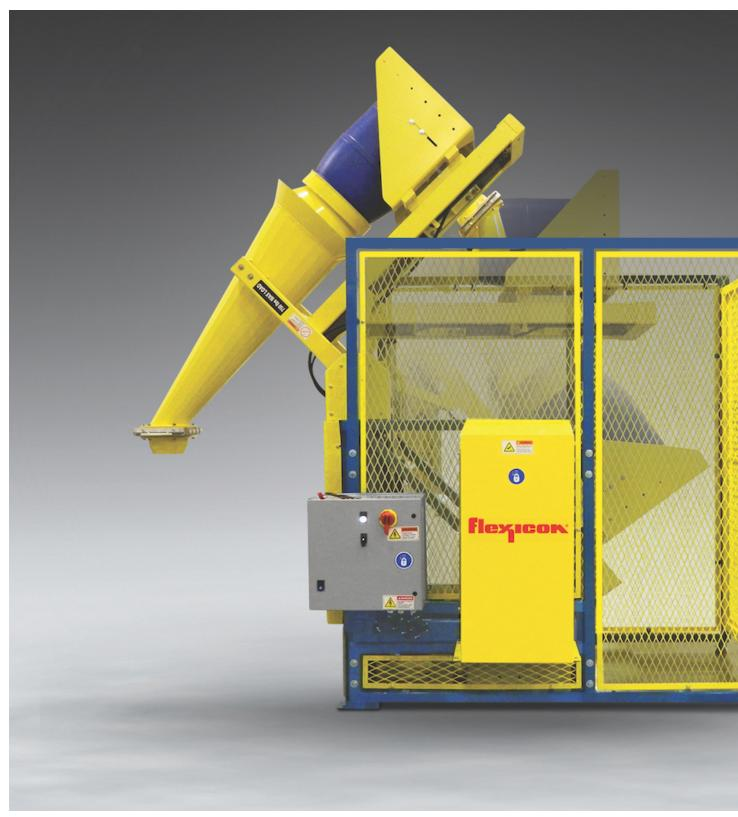
An all-new TIP-TITE® Drum Tipper with elongated discharge cone seals the drum rim before tipping the drum, seating the spout of the discharge cone against a gasketed receiving ring on vessel lids for dust-free discharging.
