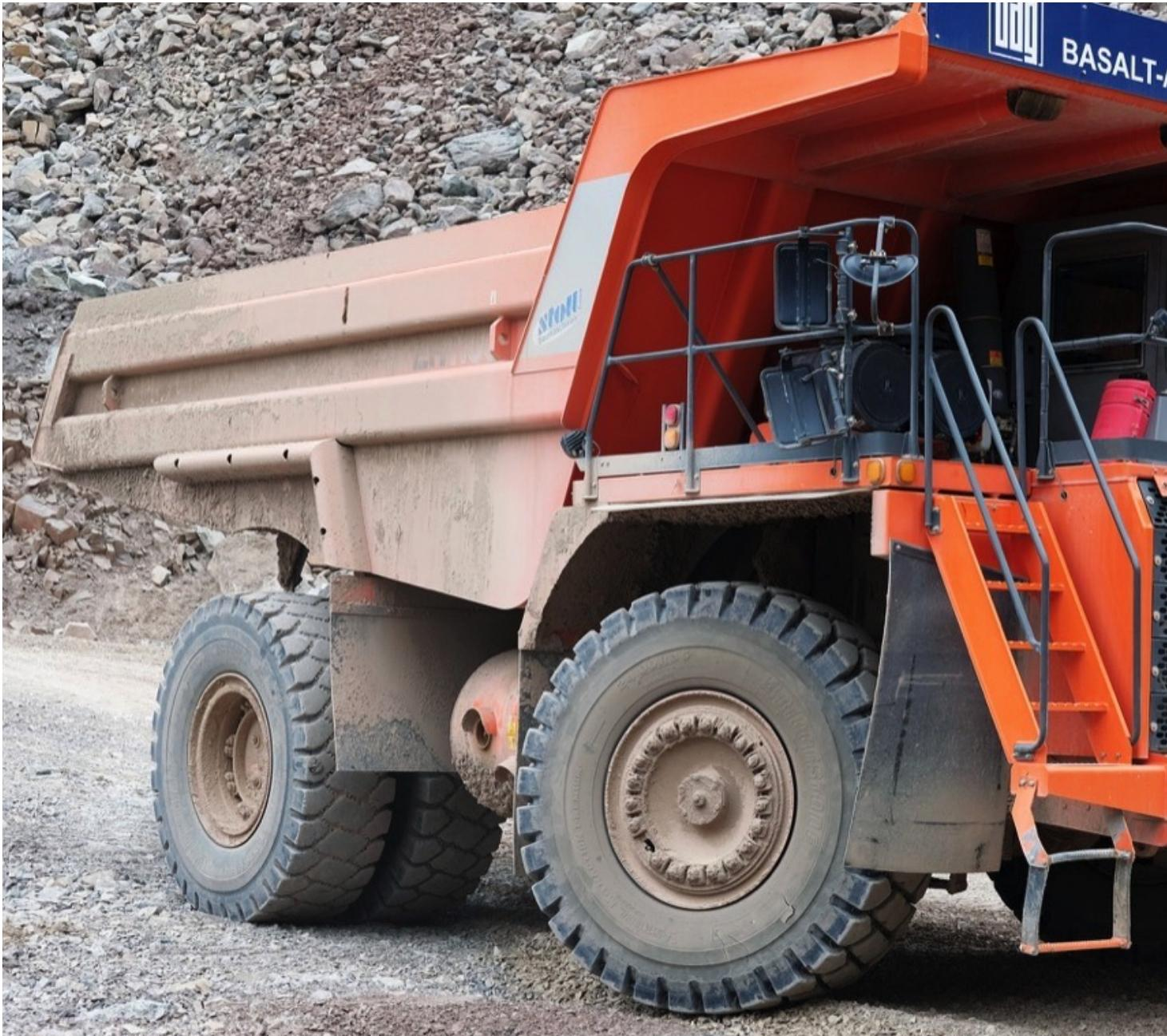
The "Kuselit" microdiorite is transported after blasting with big dump trucks to the primary gyratory crusher.
