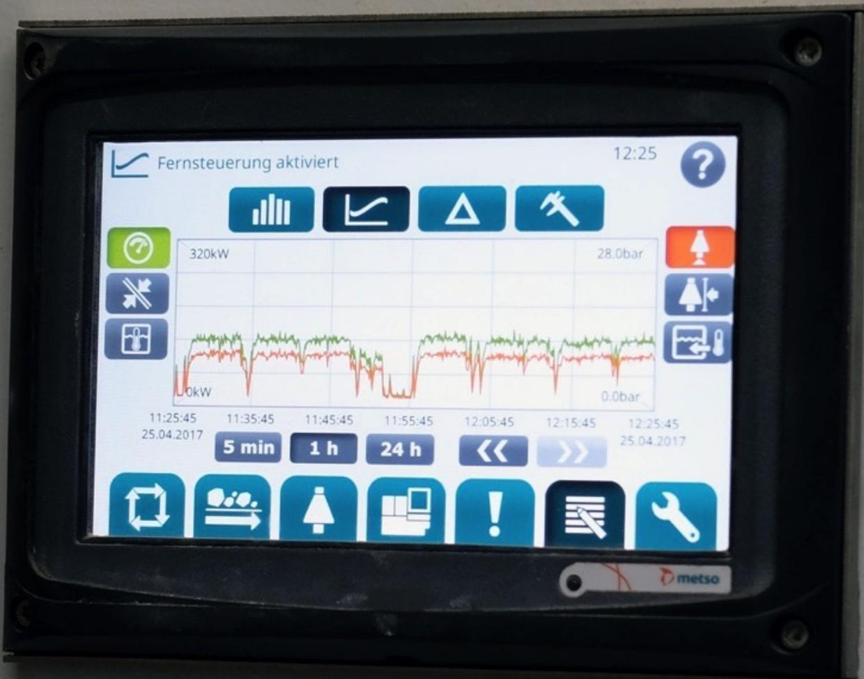
The Metso IC50 process steering with informative four colour display makes all crusher adjusting safe and easy.
