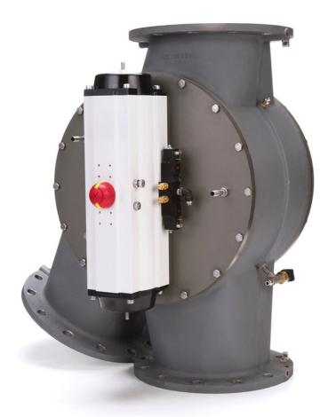
To complete the unit, a pneumatic actuator providing a 4 second actuation time between ports, a 4-way double, and 3-way single solenoid air control valve with NEMA 4 enclosure, and 2 SPST proximity sensors are included. The new version of the PST30 Diverter Valve can also be designed without inflatable seals.
