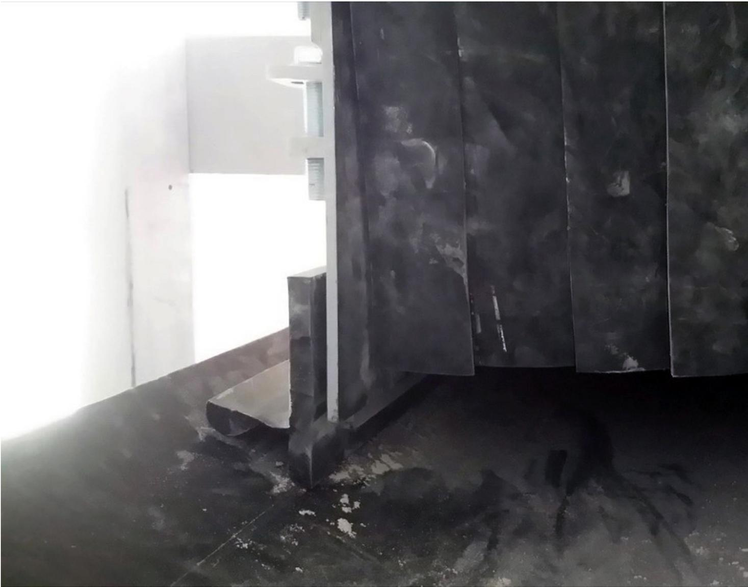
Dust curtains slow down the air flow and reduce fugitive particle emissions.
