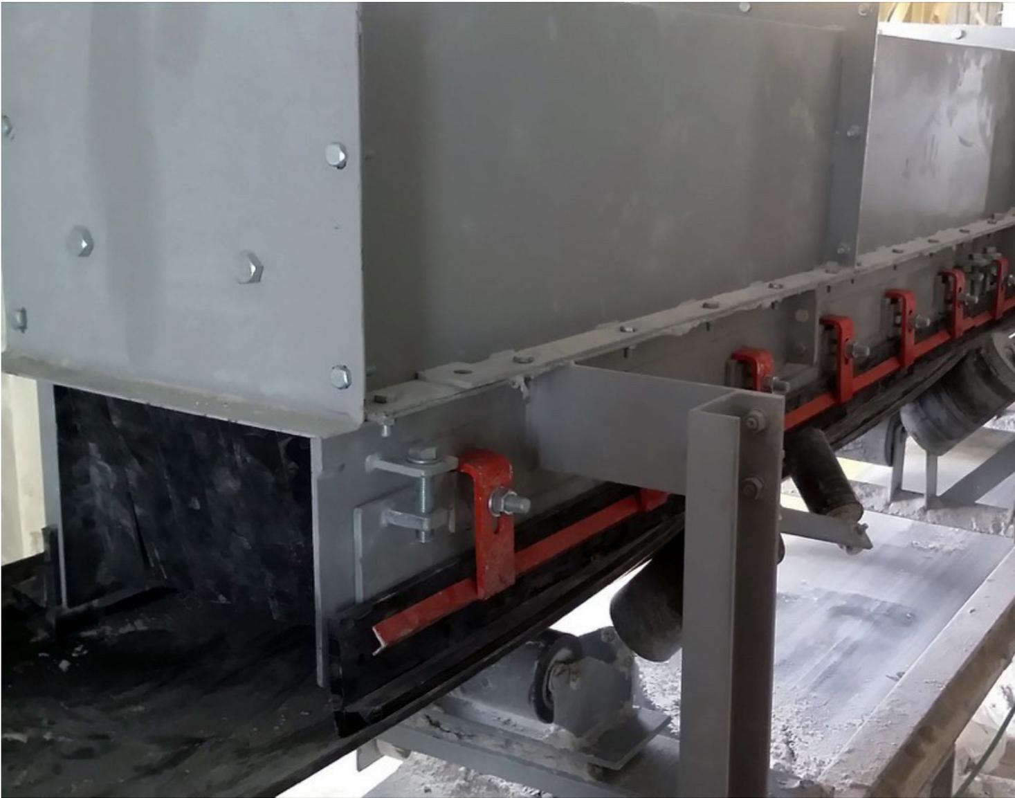
The external wear liner and apron seal help prevent damage to the chute wall.
