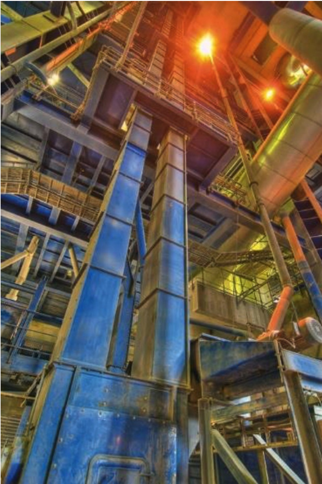
Example of a BWZ AUMUND chain bucket elevator (picture: Aumund)
