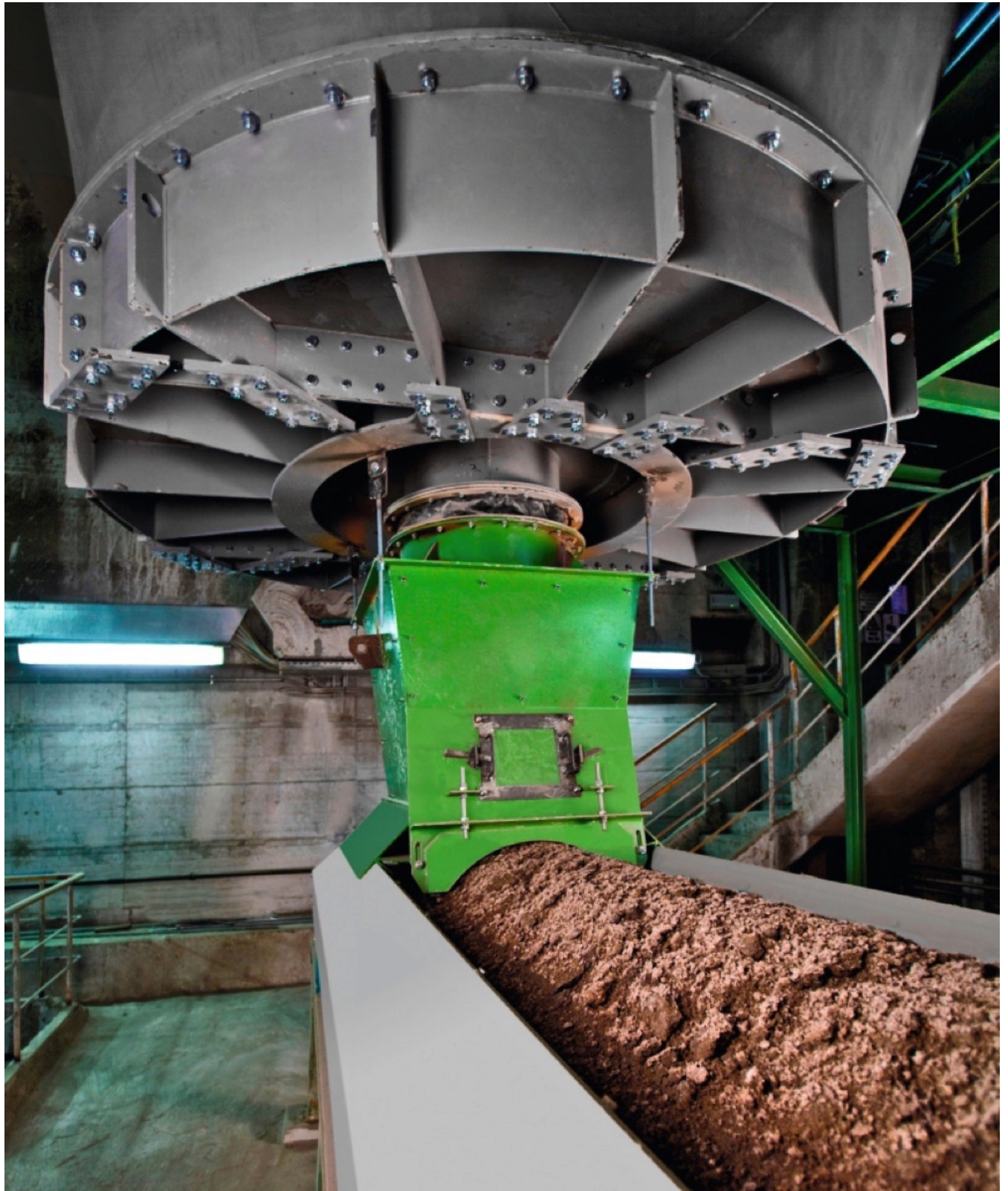
Two CENTREX machines will be extracting a mixture of limestone and clay as well as iron ore from silos. (Picture: AUMUND)
