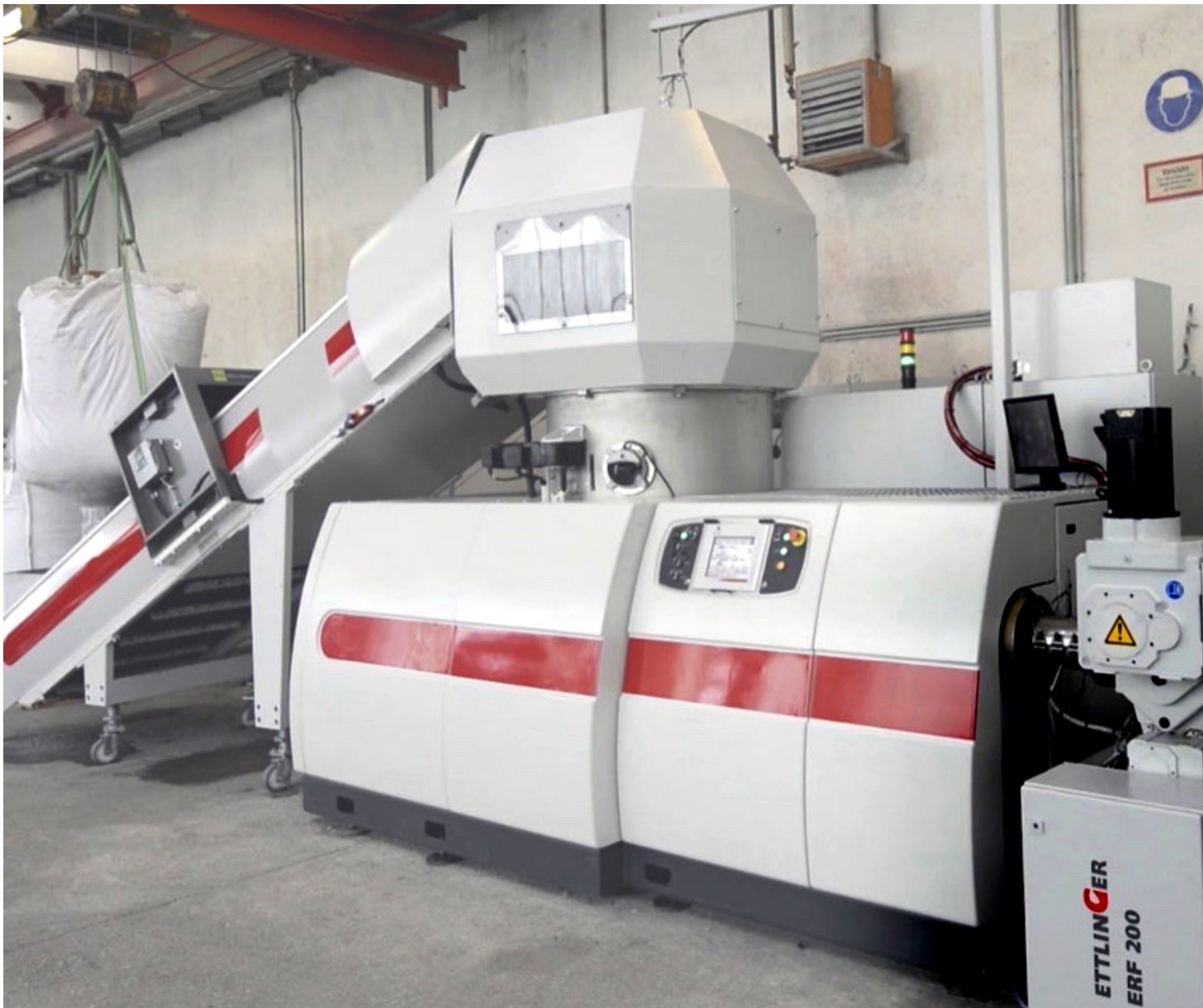
The ETTLINGER ERF 200 high performance melt filter on an extrusion line at CANDI is used to process industrial plastic waste containing 10% or more aluminum or paper. (Picture: ETTLINGER)
