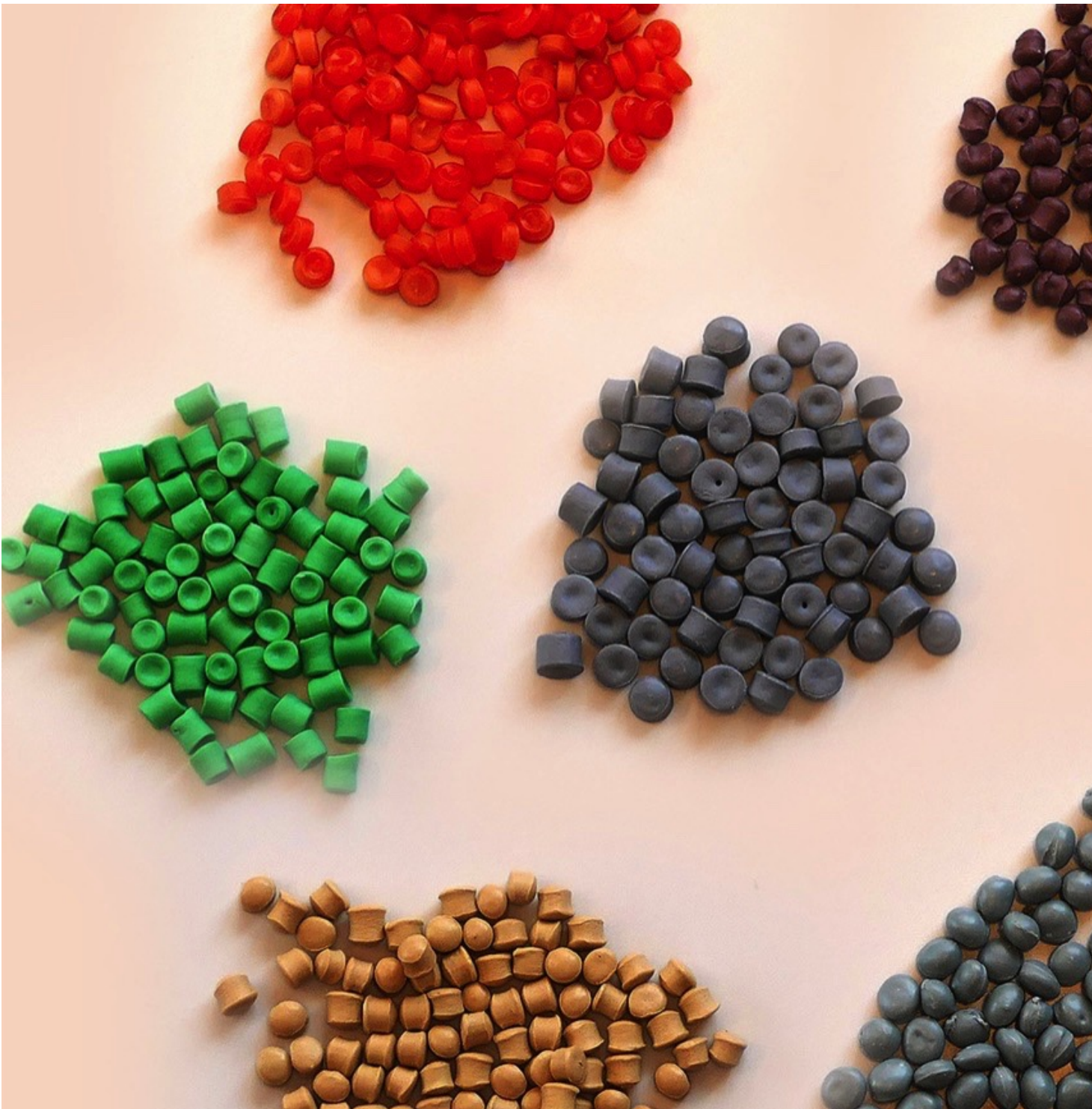
CANDI regrind: PP from colored and transparent ketchup bottles (orange), PE / PP compound (green and blue), PP from Kinder eggs (beige), PS from yogurt pots (light gray), PS from coffee cream packets (brown), HDPE from multilayer material for bottled liquid dairy products (dark gray). (Picture: ETTLINGER)
