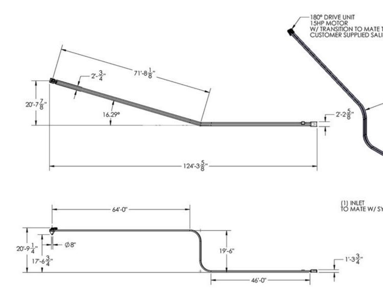
Circuit length is 282 ft (approx. 86 m) with a hardened steel chain and split UHMW pucks.
