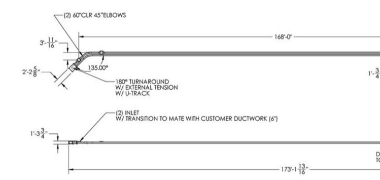
Circuit length is 348 ft (approx. 106 m) with hardened steel chain and split UHMW pucks.
