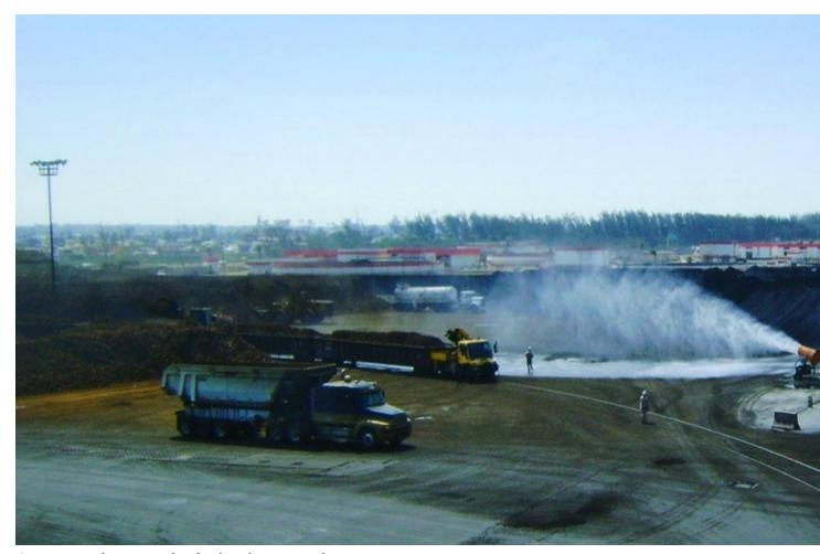
As operations and winds change, the cannons can be easily relocated and readjusted.
