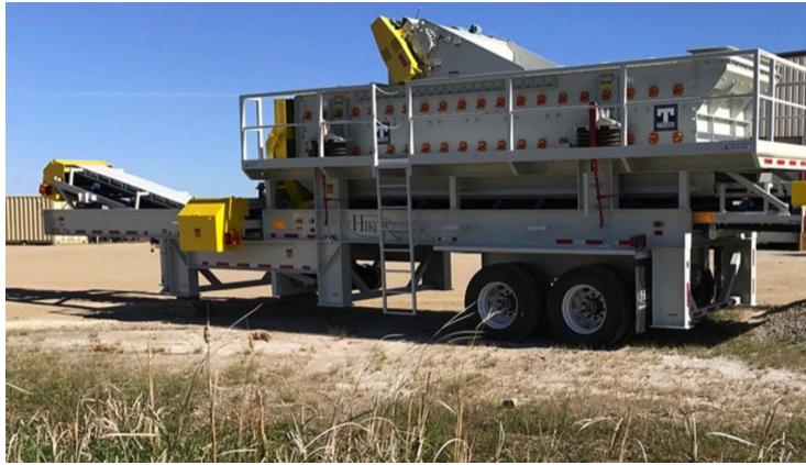
Haver & Boecker Portable L-Class; the compact machine is versatile and easy to maintain, with no timing belts or gears that normally need replacing.
