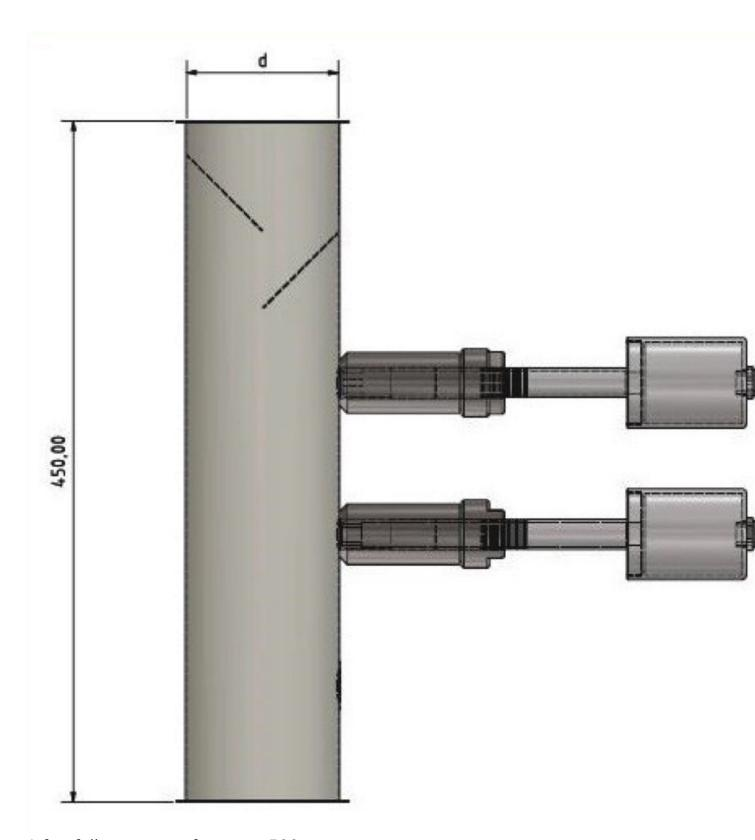
A freefall structure of approx. 500 mm is required for successful measurement.
