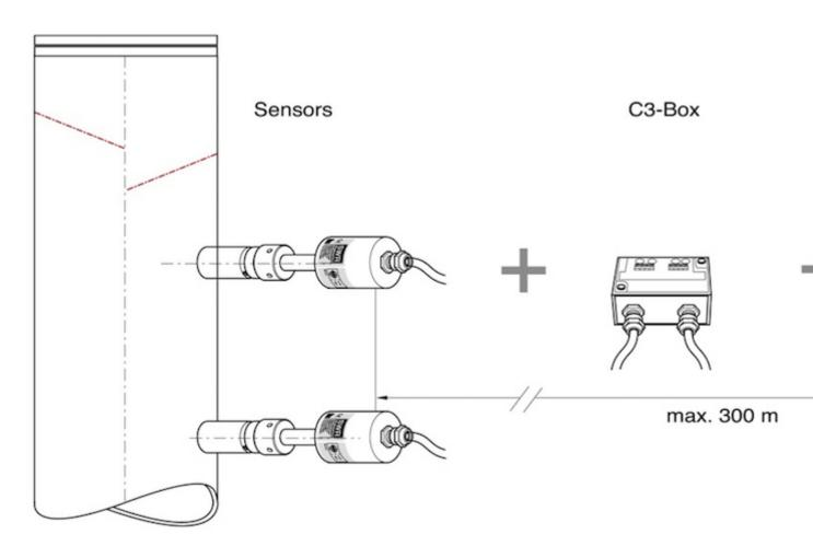
The sensors are connected to an evaluation unit via a C3 box.
