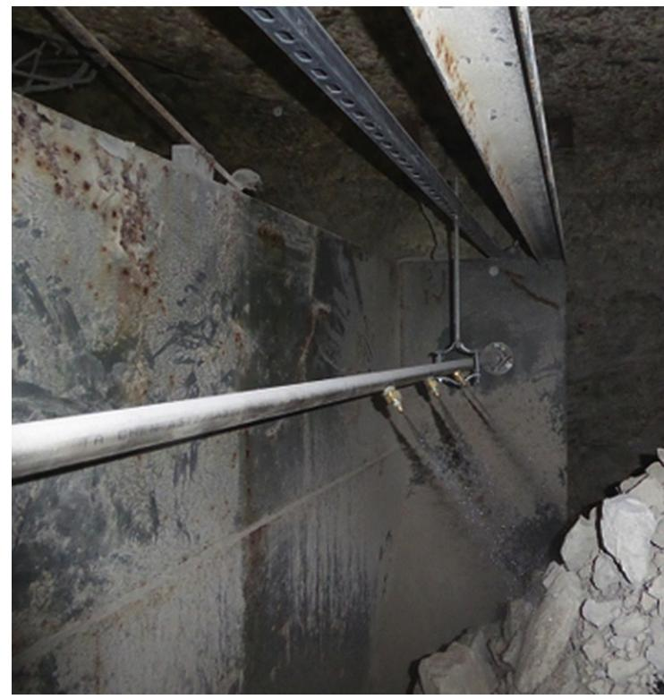
The dust management system treats the material from the top and bottom during discharge.
