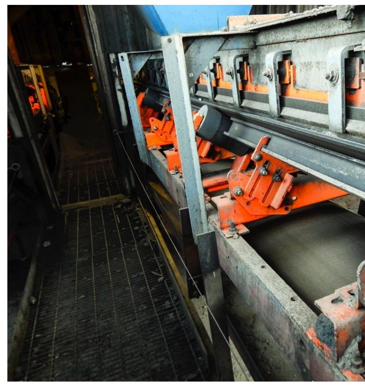
Technicians installed three impact cradles in the loading zones on each conveyor to create a flat edge for improved containment.
