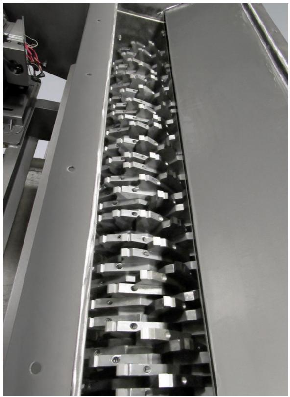
Each of 72 holders secures four 25 mm-wide tungsten carbide cutter tips (total 288 tips) to continuously shear oversize materials against twin, stationary bed knives. The infeed throat accepts bulk materials up to 1830 x 572 mm in size.
