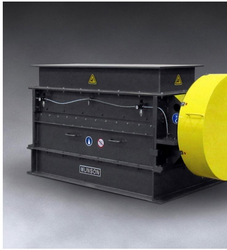
New Magnum72-AR Screen Classifying Cutter reduces up to 20.4 m3/h of abrasive bulk material into controlled particle sizes from 102 mm to 3.2 mm in diameter with little or no fines and virtually no heat generation.
