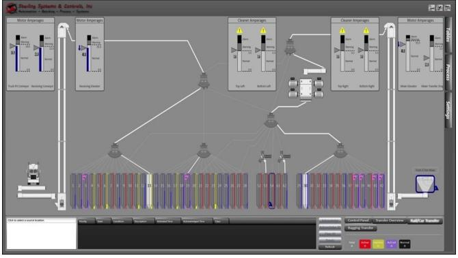
Truck or Railcar transport can be accommodated. Feed rates are controlled to maximize efficiency and safety. After the material has been moved into the containment location (bin etc.) the system logs and weighs empty trucks before they leave the facility. Weight measurements, before and after material transfer, are logged into the tracking function, maintaining accuracy and traceability.
