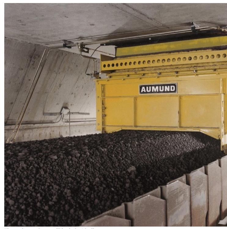
The order package will include 19 silo discharge gates which will be installed under the clinker silo. (Photo: AUMUND)
