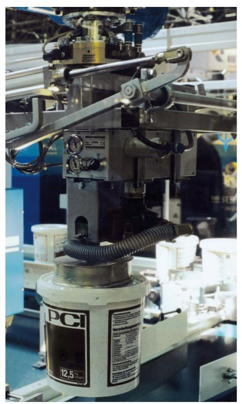
The gripper is specially designed to handle all items with surfaces that need to be suctioned.
